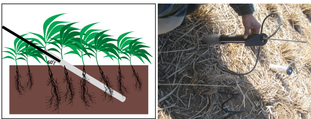
(a) Minirhizotron imaging system illustration (b) Minirhizotron imaging system in field
